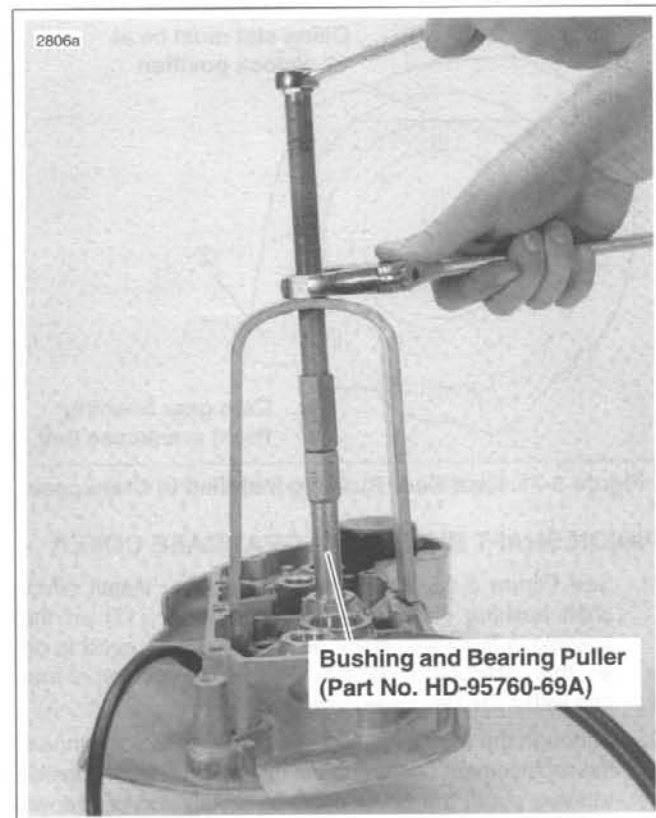
Figure 3-69. Removing Bushing
