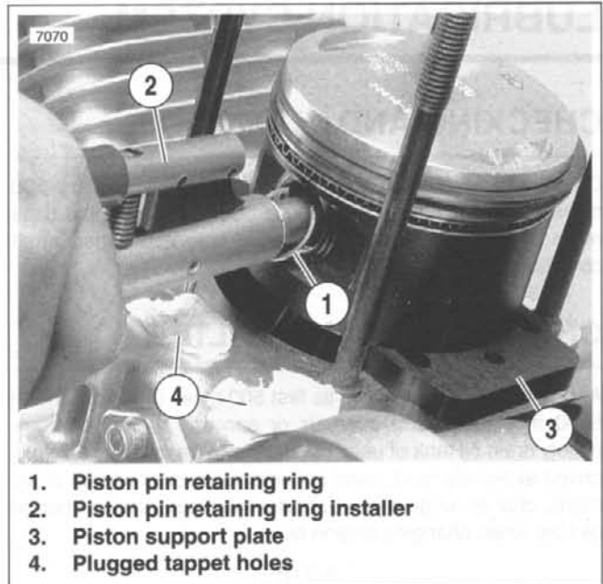
Figure 3-42. Installing Piston Retaining Rings
