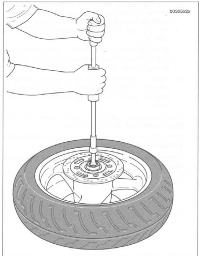
Figure 2-15. Removing Wheel Bearing
