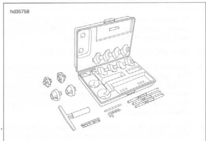
Figure 3-22. Valve Seat Cutter
