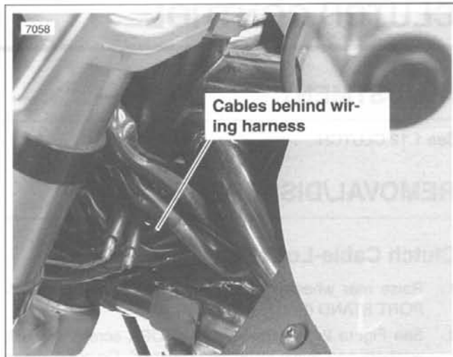
Figure 2-129. Steering Neck Routing
