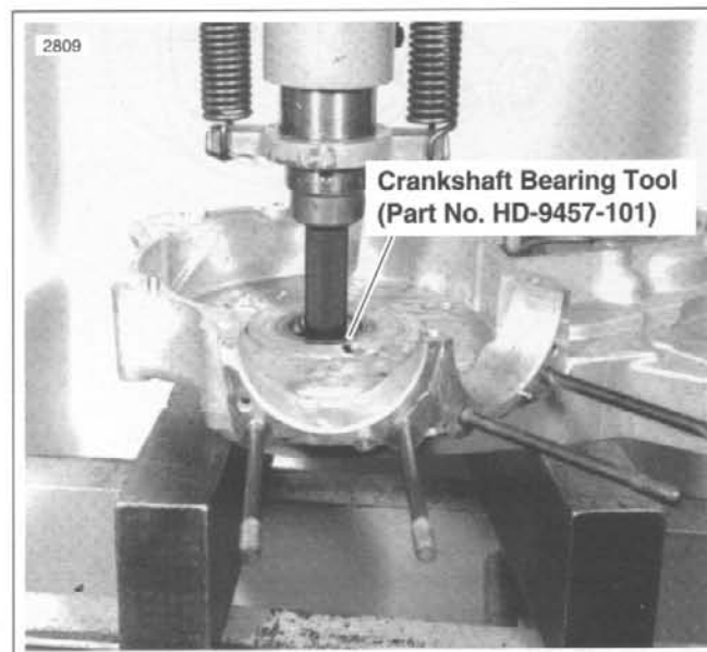
Figure 3-98. Sprocket Shaft Outer Race Removal
