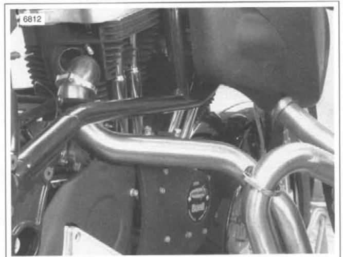
Figure 2-145. Exhaust Header Alignment
