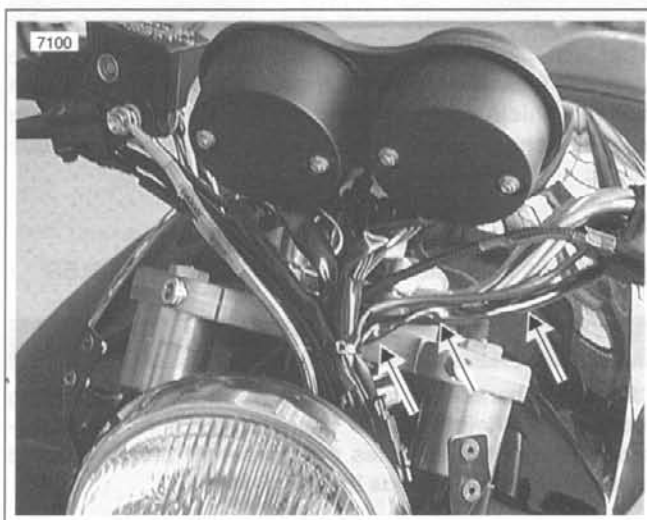
Figure 7-57. Routing Handlebar Wires, Left
