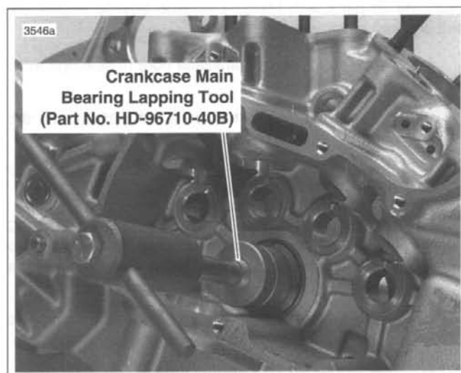
Figure 3-139. Lapping Pinion Shaft Main Bearing
