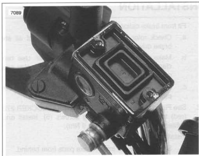
Figure 2-40. Front Master Cylinder Gasket
