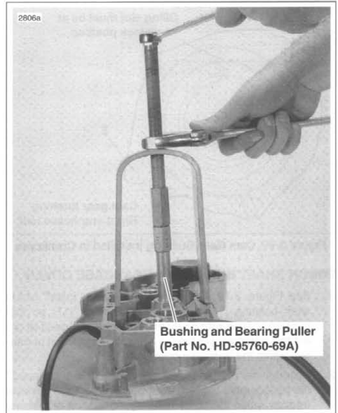
Figure 3-83. Removing Bushing
