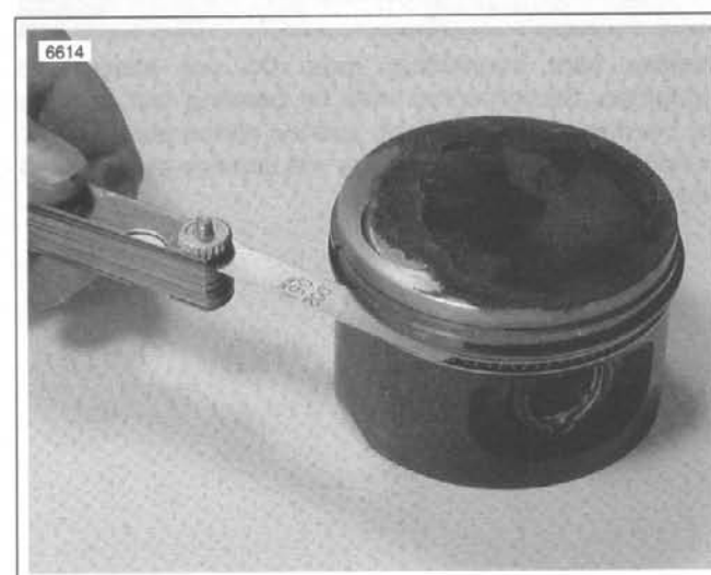
Figure 3-39. Measuring Ring Clearance in Groove
