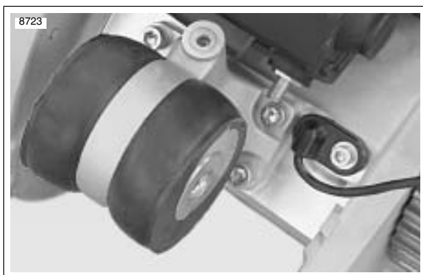
Figure 6-48. Rear Isolator Assembly
