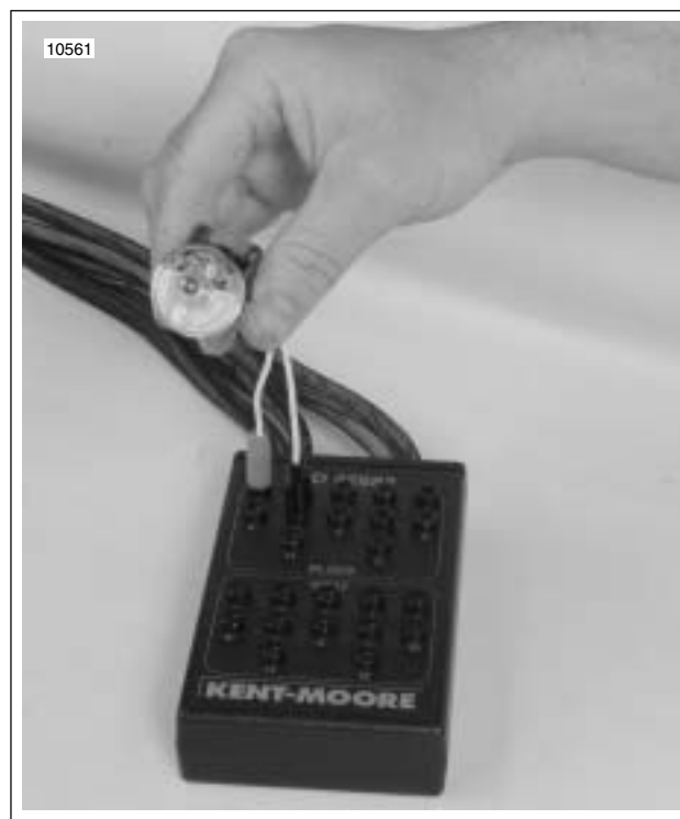
Figure 4-48. Testing Ignition Coil Connectors
