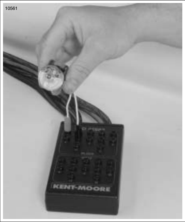
Figure 4-19. Ignition Coil Circuit Test
